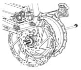
5. Mount the 4mm washer on both sides of the frame.
