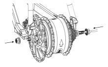
7. Mount the shaft end sheath on both sides of the shaft ends.
