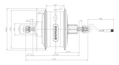
OLD: 175mm Shaft length: 235mm Motor cable length: L=250mm
