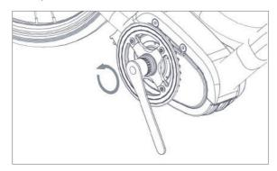
Using the special tool provided, tighten the locking nut onto the axel.
